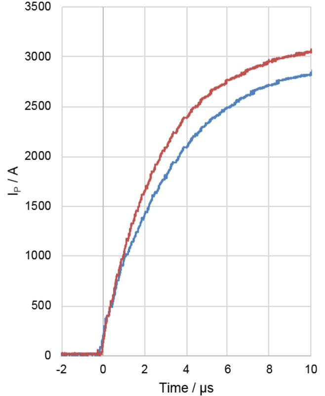
Fast increasing currents (higher than the specified  $I_{P,max}$ ), e.g. in case of a short circuit, can be transmitted because the currents are transformed directly and be limited by diodes only.
